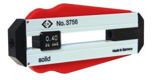
Features & Benefits  $\sim$  Compact precision wire strippers for repeatable, damage free stripping of PVC, Teflon & similar coated wire  $\sim$  Graduated depth stop for stripping to precise lengths  $\sim$  Specially hardened blades for outstanding long term performance  $\sim$  50 mm scale with 1 mm graduations and length stop  $\sim$  For diameter: 0,80 mm (20 AWG)
